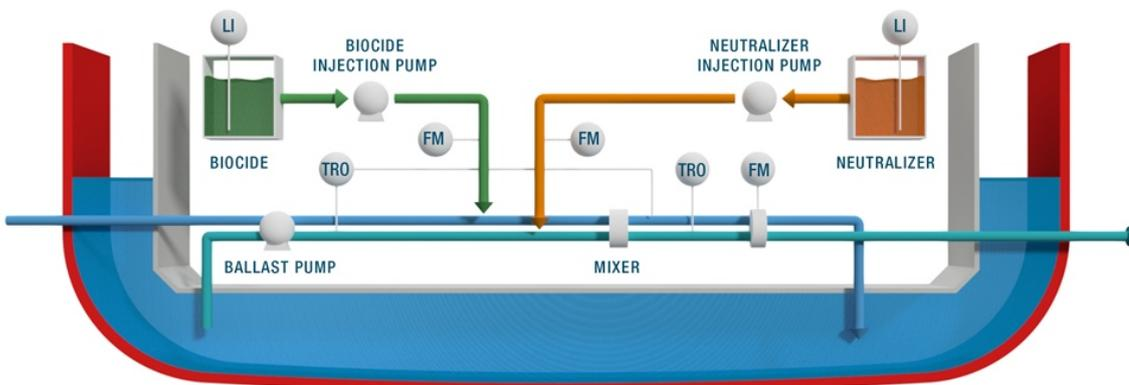
LI = LEVEL INDICATOR FM = FLOW METER TRO = TOTAL RESIDUAL OXIDANT
